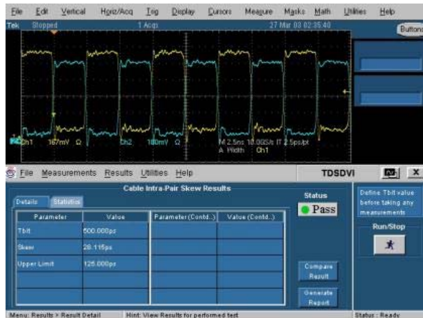
Figure 3-163: Cable Intra-Pair Skew results
